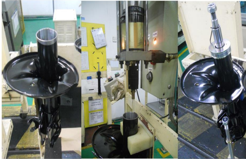
Figure 2. MR fluid damper assembly.
