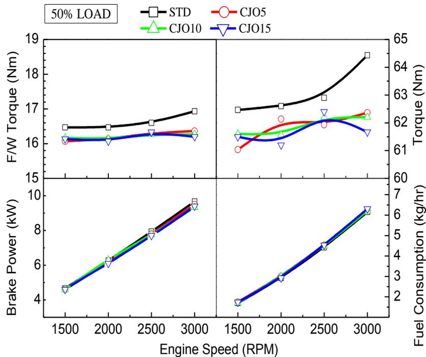
Figure 6. Effects of engine speed on performance under different blending ratios with medium load (50% load condition).
