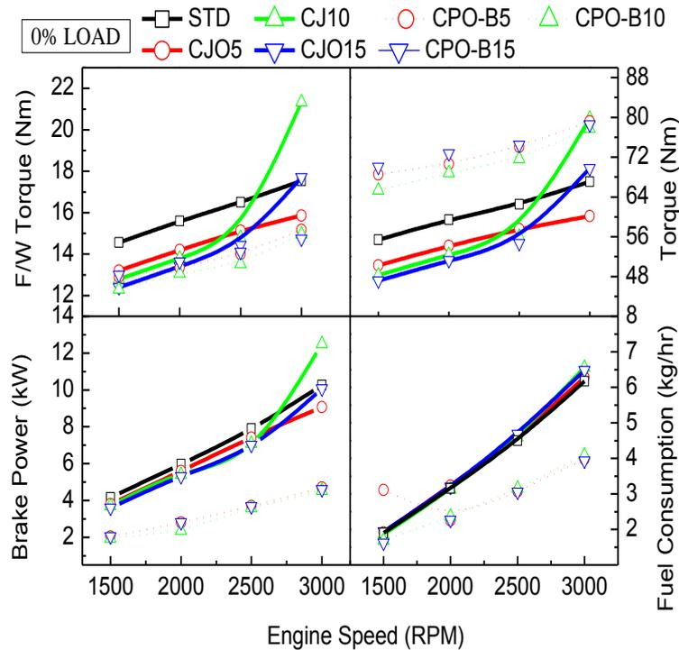
Figure 8. Effects of engine speed on performance under different blending ratios without load conditions.
