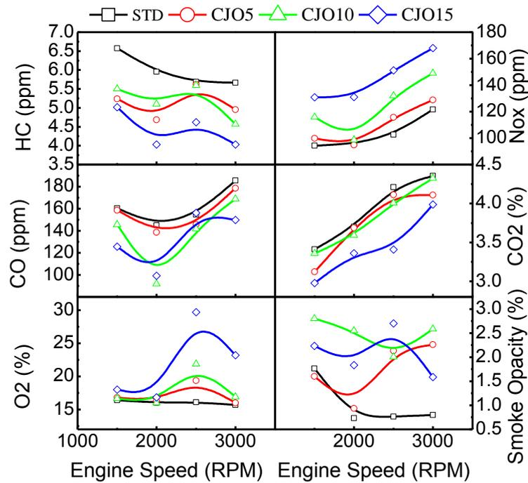
Figure 5. Effects of engine speed on emissions under different blending ratios with medium load (50% load condition)
