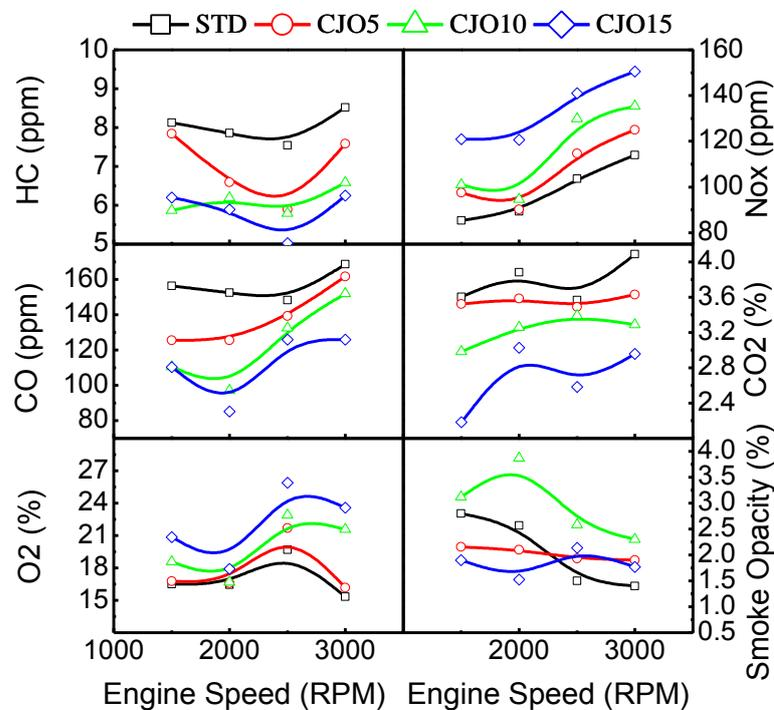
Figure 3. Effects of engine speed on emissions under different blending ratios without load condition.
