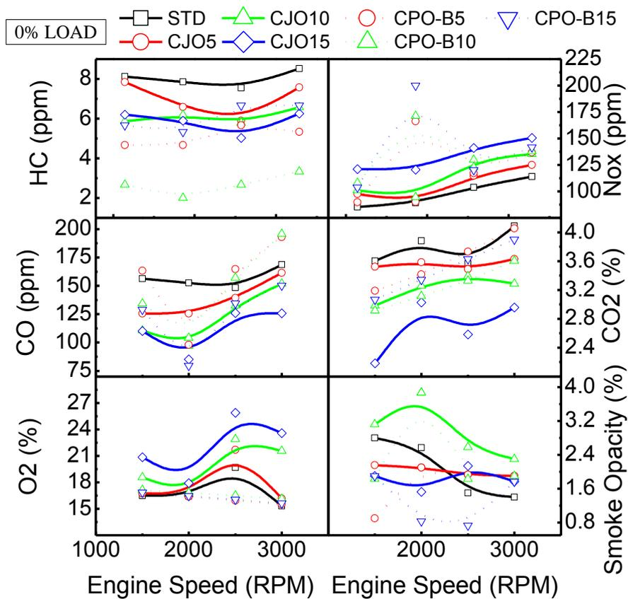
Figure 7. Effects of engine speed on emissions under different blending ratios without load conditions.
