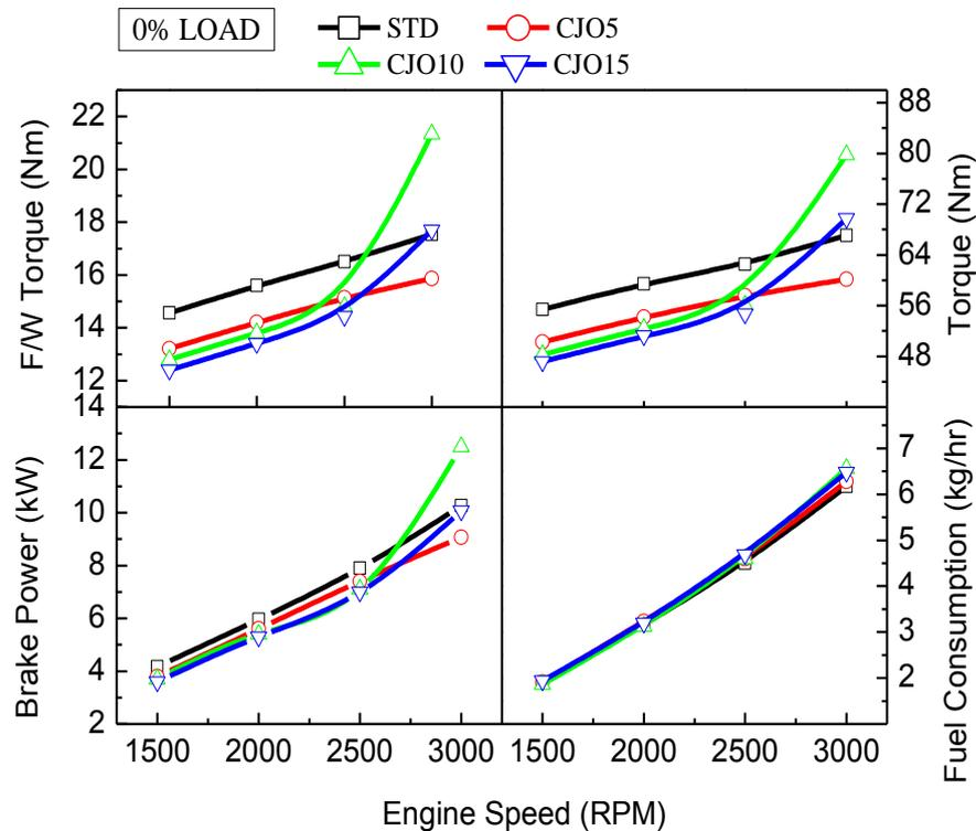
Figure 4. Effects of engine speed on performance under different blending ratios without load conditions
