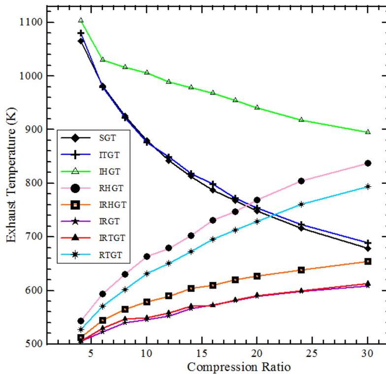
Figure 3. Effect of compression ratio on the exhaust temperature of the gas-turbine plants.
