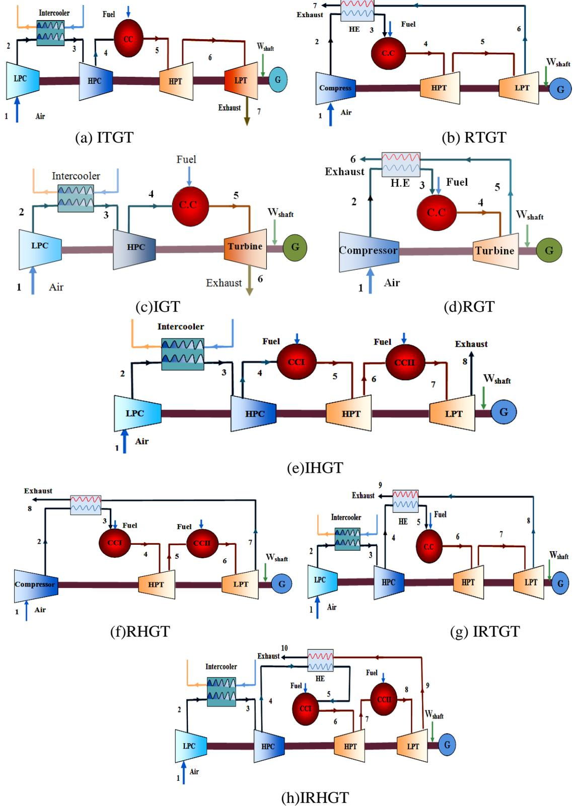
Figure 1. Configurations of gas turbine performance enhancing strategies.
