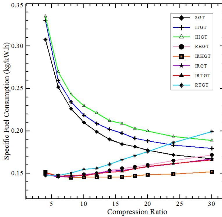
Figure 5. Variation of compression ratio on the specific fuel consumption of the gas-turbine plants.
