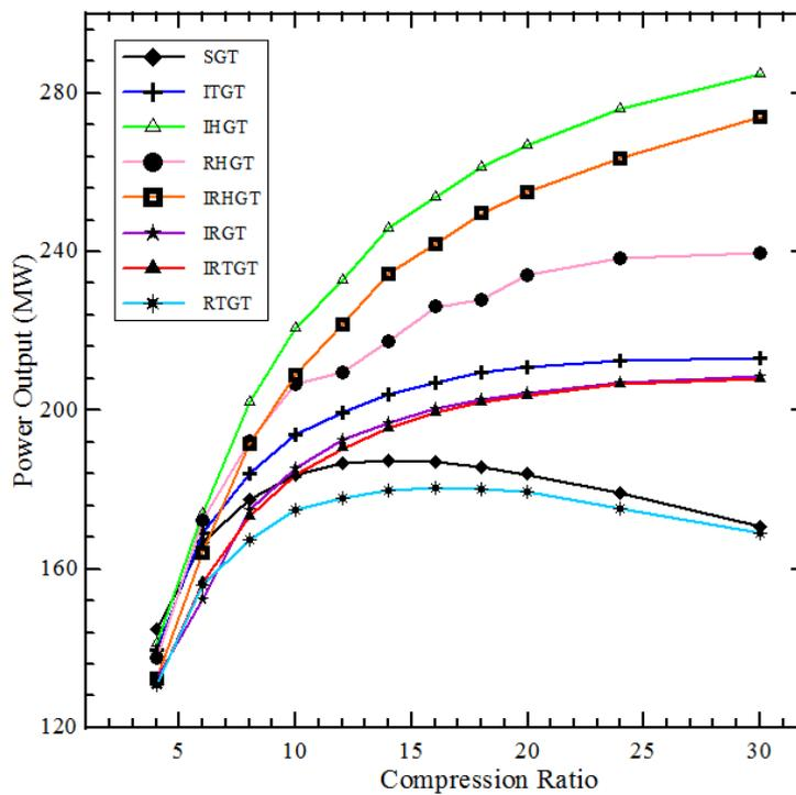
Figure 6. Effect of variation of the compression ratio on the power output of the gas-turbine plants.
