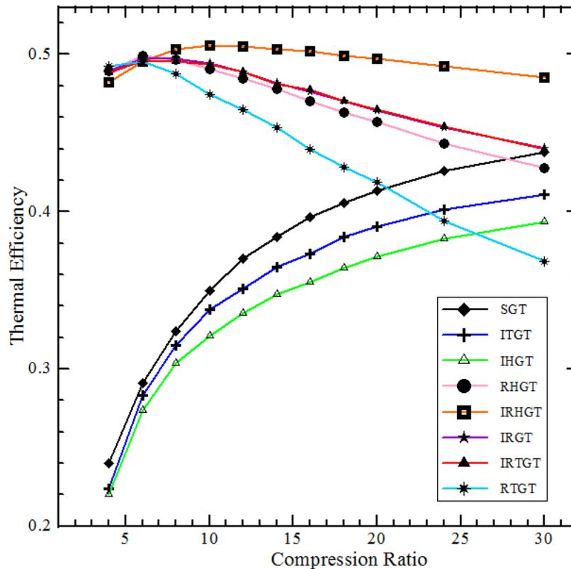
Figure 4. Effect of compression ratio on the thermal efficiency of the gas-turbine plants.
