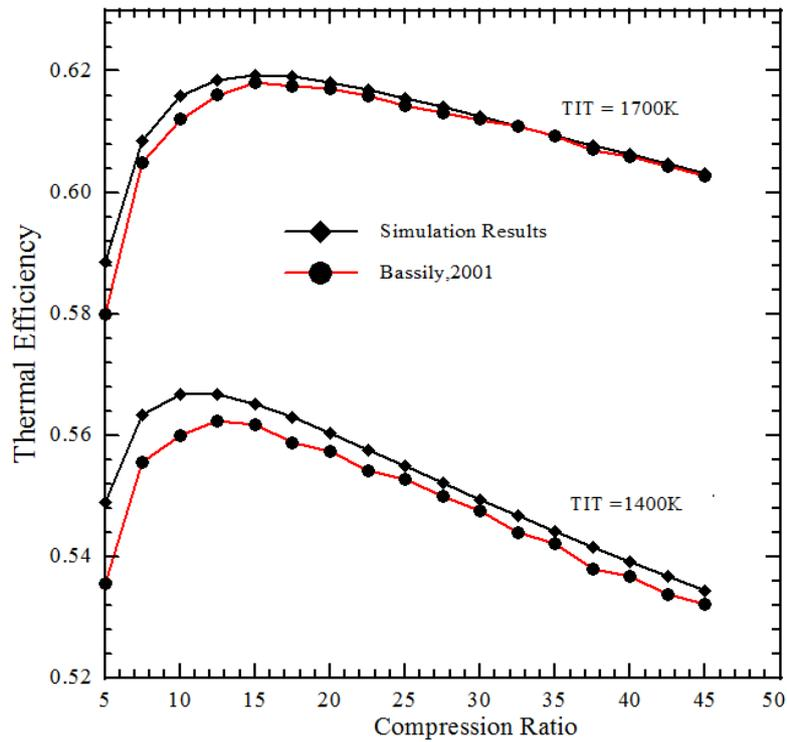
Figure 2. Comparison between simulated thermal efficiency of the intercooler-regenerative-reheat gas turbine and Bassily model with the effect of the compression ratio.
