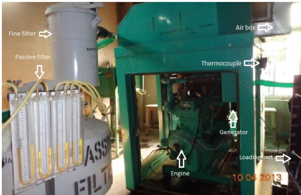
Figure 3. Photograph of the test engine setup with gasifier
