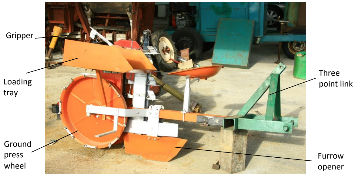
Figure 3. Major components of the mechanical transplanter
