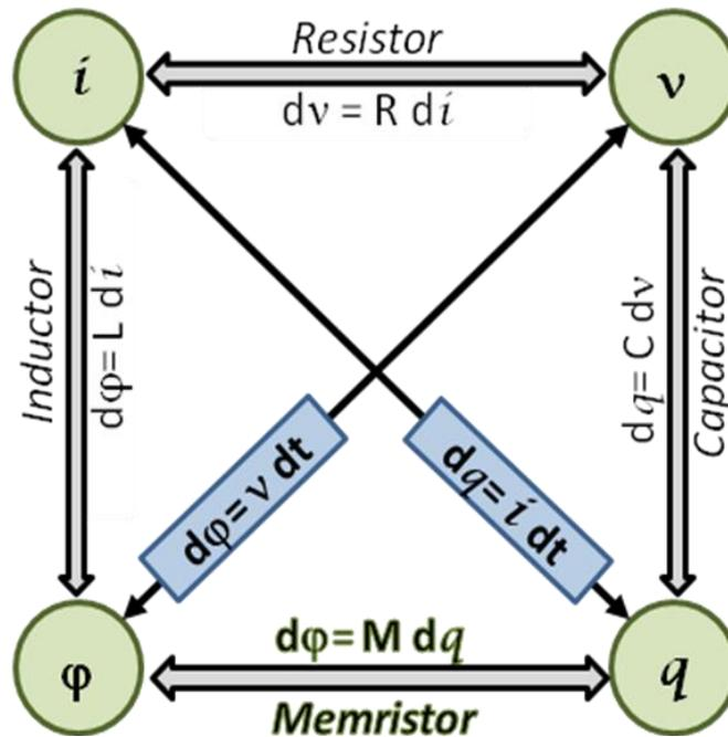
Figure 1. Leon Chua's symmetrical argument showing that a memristor completes the four fundamental passive circuit elements (Chua, 1971).
