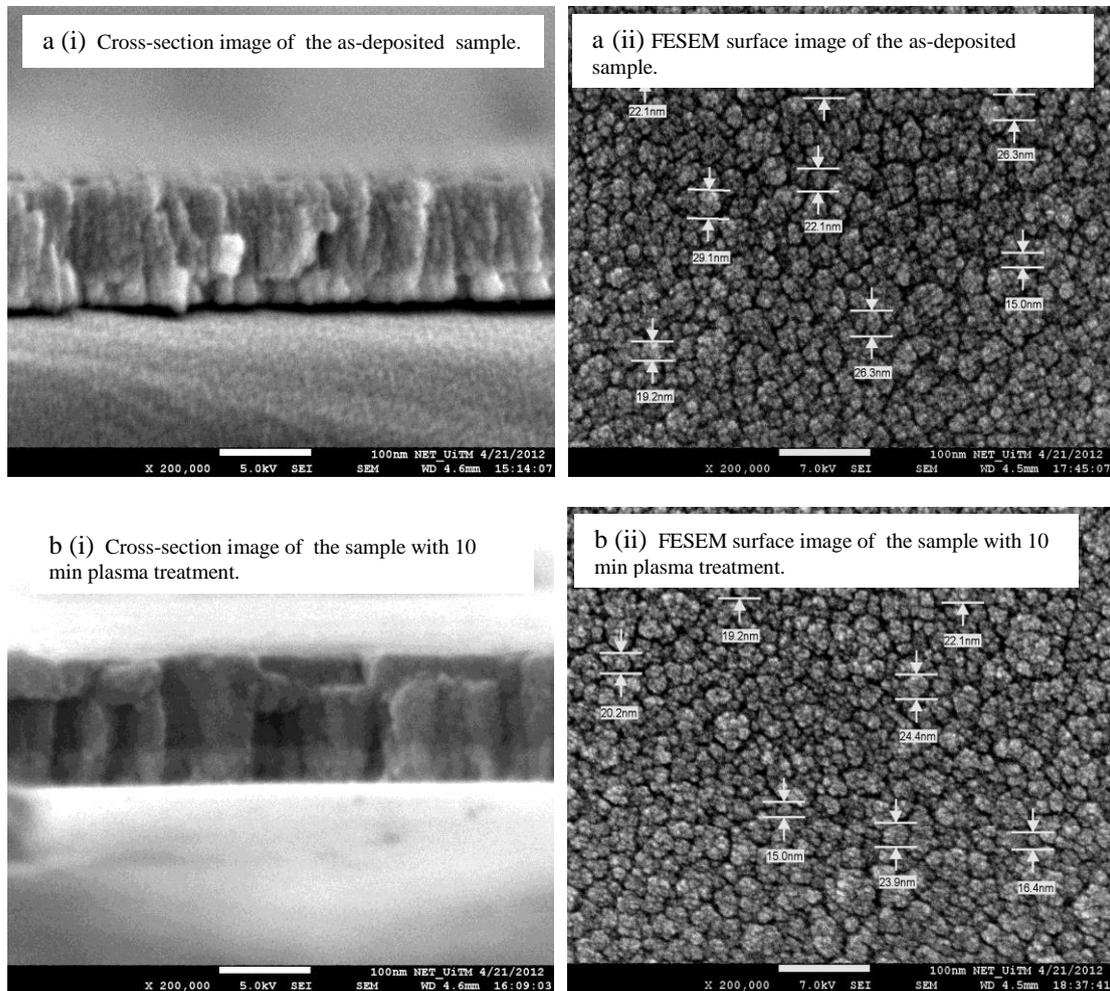
Figure 4. (a) As-deposited sample, (b) Sample with 10 min plasma treatment.
