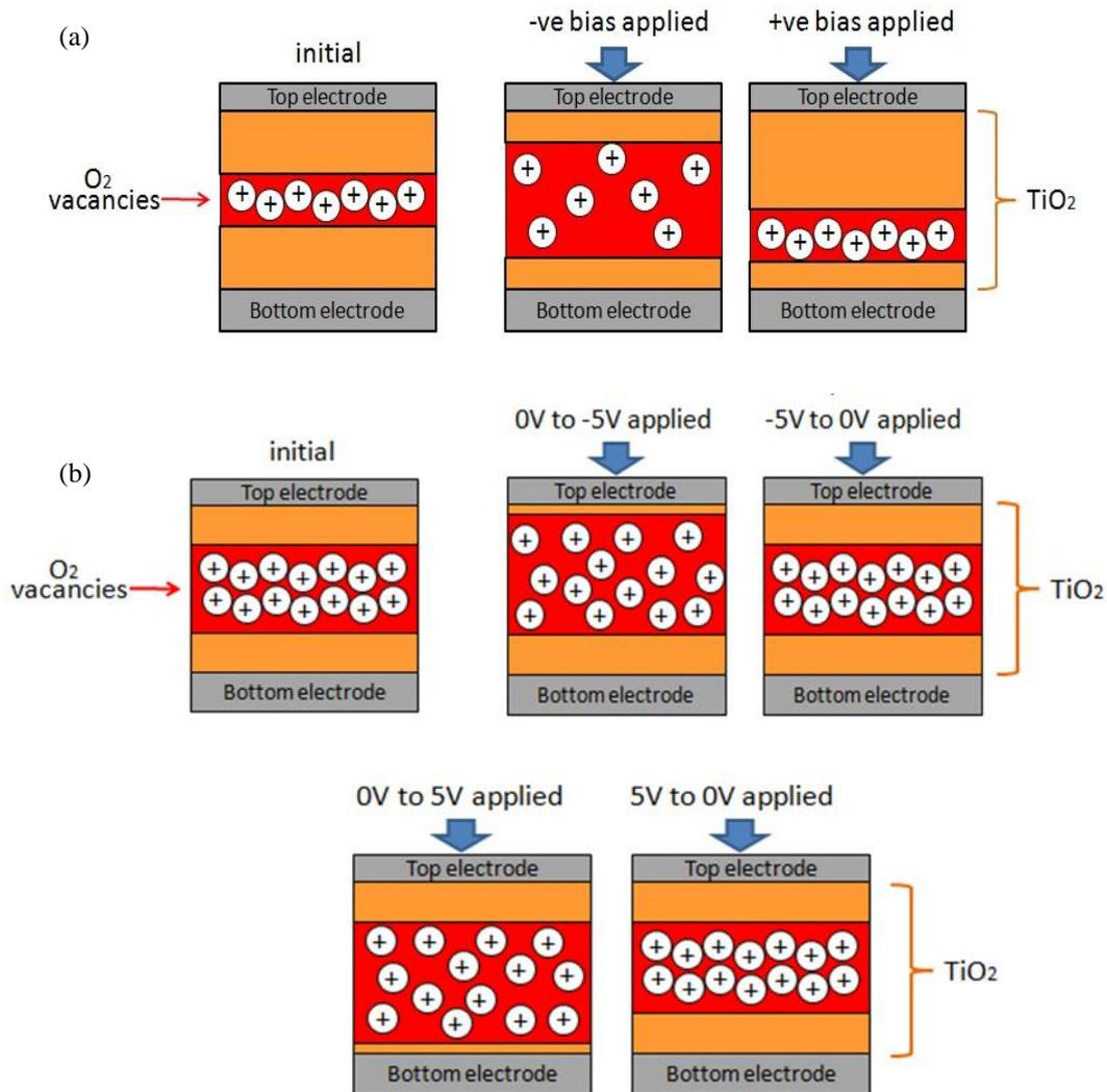
Figure 3. Schematic diagram of possible ionic (oxygen vacancies) movement for (a) as-deposited sample, and (b) sample with 10 min plasma treatment. The thickness of the titania active layer is drawn excessively thickly for a clearer view and is thus not to scale.
