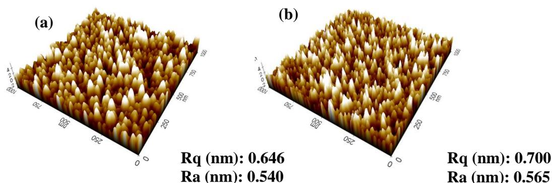
Figure 5. The 3-dimensional AFM image and surface roughness of the titania thin film exposed to plasma treatment: (a) as-deposited sample; (b) sample with 10 min plasma treatment.
