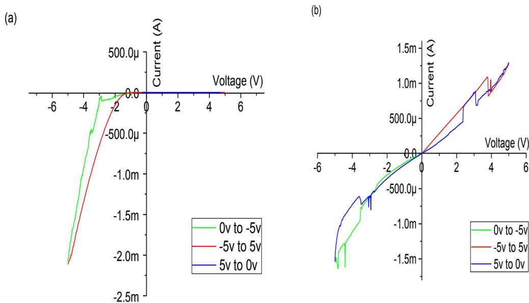
Figure 2. Memristive switching curves experiential from the current-voltage (I-V) measurement system which was measured from the voltage loop 0V→-5V→5V→0V 5V→5V→ -5V: (a) as deposited sample (b) 10 min plasma treatment.
