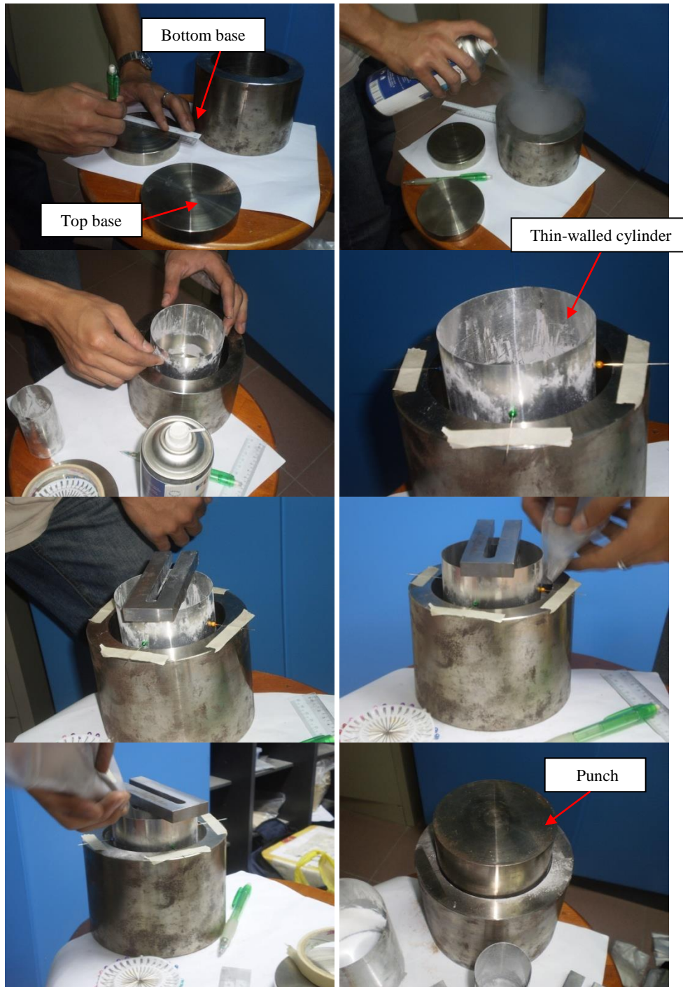
Figure 3. Stacking powders mixture into die.
