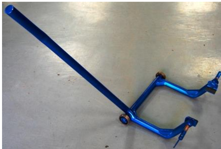
Figure 10. Frame of the superbike paddock stand after welding.
