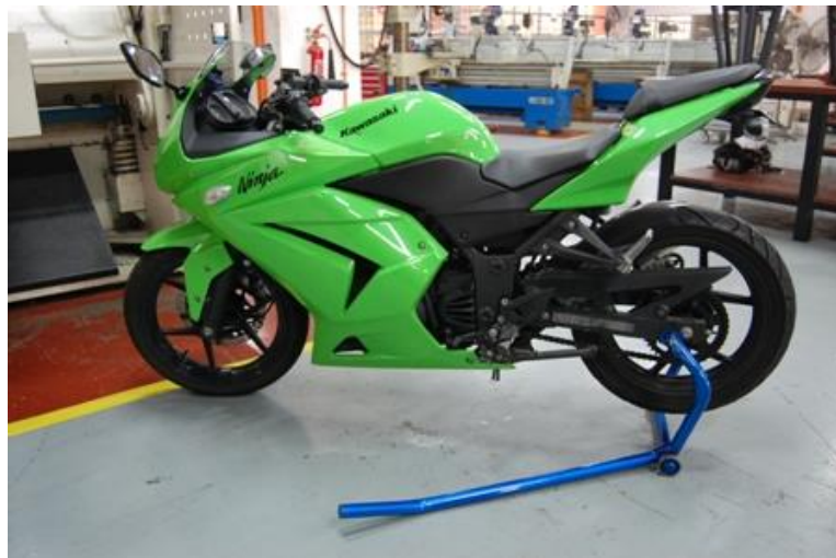
Figure 14. The superbike paddock stand with superbike's rear tyre lifted.
