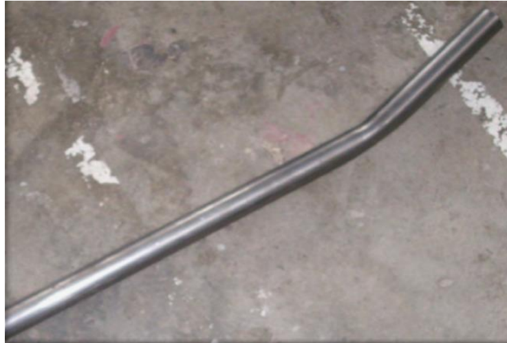
Figure 9. Handle of the superbike paddock stand after bending.
