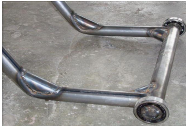
Figure 10. Frame of the superbike paddock stand after welding.
