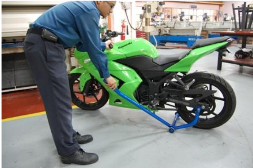
Figure 13. Single user demonstration of superbike paddock stand use.
