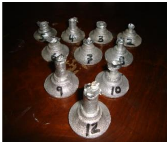
Figure 3. Aluminium alloy casting at different shell wall thicknesses
