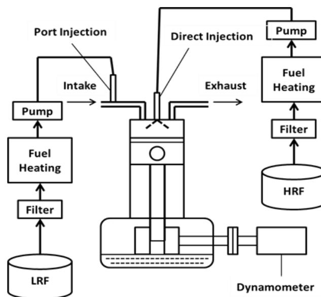
Figure 5. Experimental setup for RCCI with a direct and a port Injection [10].
