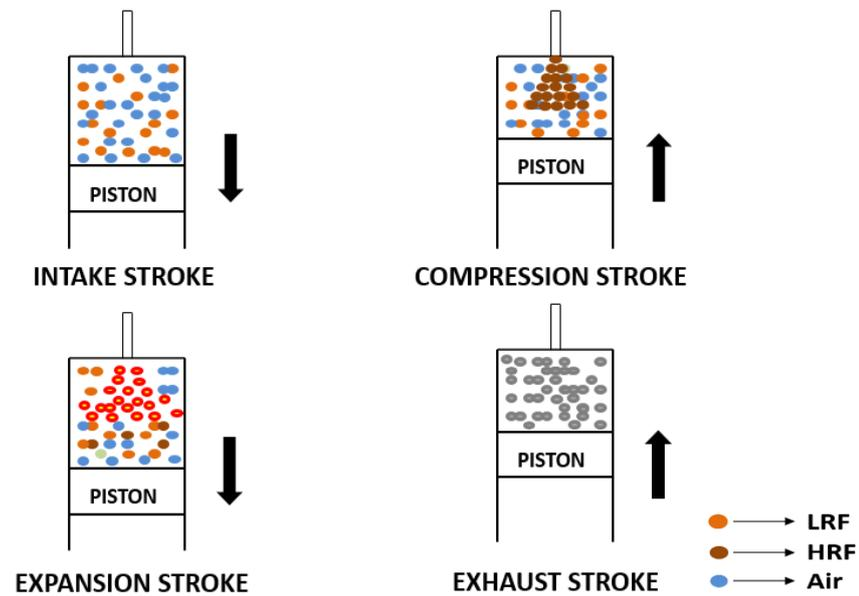
Figure 6. RCCI combustion process.
