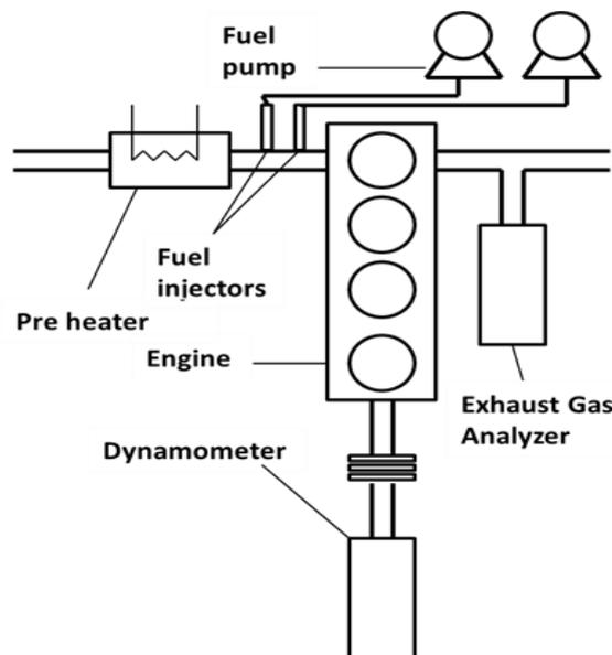
Figure 7. Experimental setup for RCCI with dual port injection [70].
