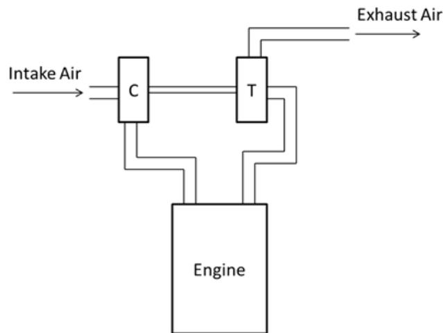
Figure 4. Turbocharging [42].
