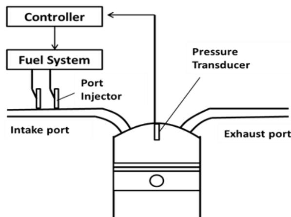
Figure 8. Experimental setup for Iso-Octane/N-heptane combination [12]
