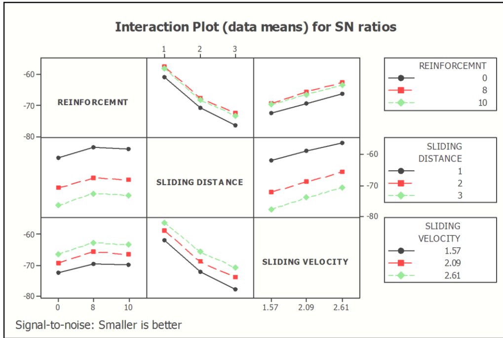
Figure 3. Interaction plot for volumetric wear rate of AA7075/TiC composites.
