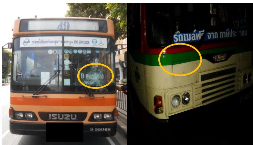
Figure 5. The low- and the high-located windshield city bus collision damage from hitting pedestrians.
