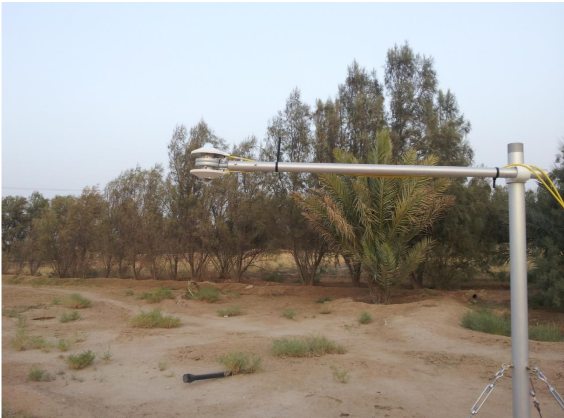
Figure 1. The pyranometer at site.
