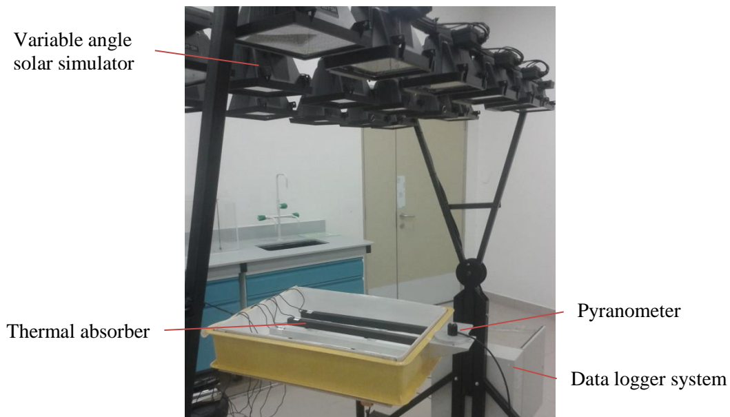
Figure 3. Experimental setup with solar simulator.
