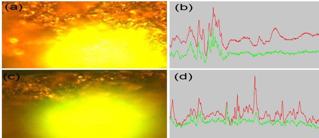
Figure 5. Typical microstructure of brass alloys with addition of various alloying elements after tensile test at Mag. 20X: (a) C38500 or CuZn39Pb3 brass alloys; (b) the bright primary phases containing alloys in C38500 on line; (c) brass type 1 alloy; (d) the bright primary phases containing alloys in brass type 1 on line.
