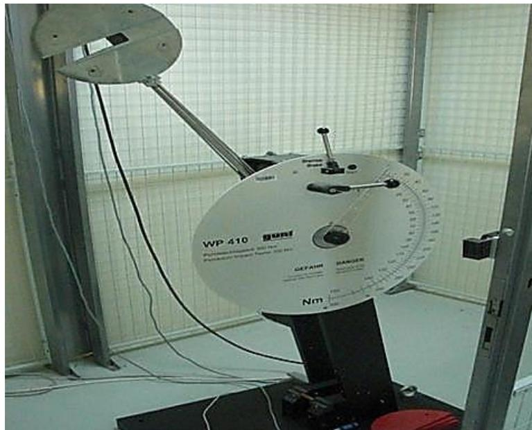
Figure 3. Equipment used for impact test.
