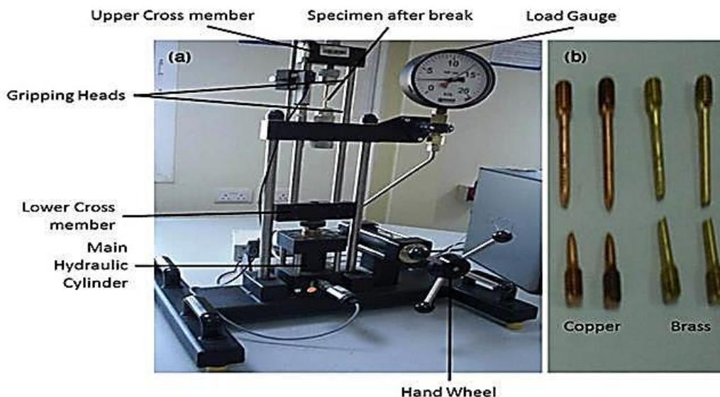
Figure 1. (a) Universal Testing Machine; (b) specimens after fracture.
