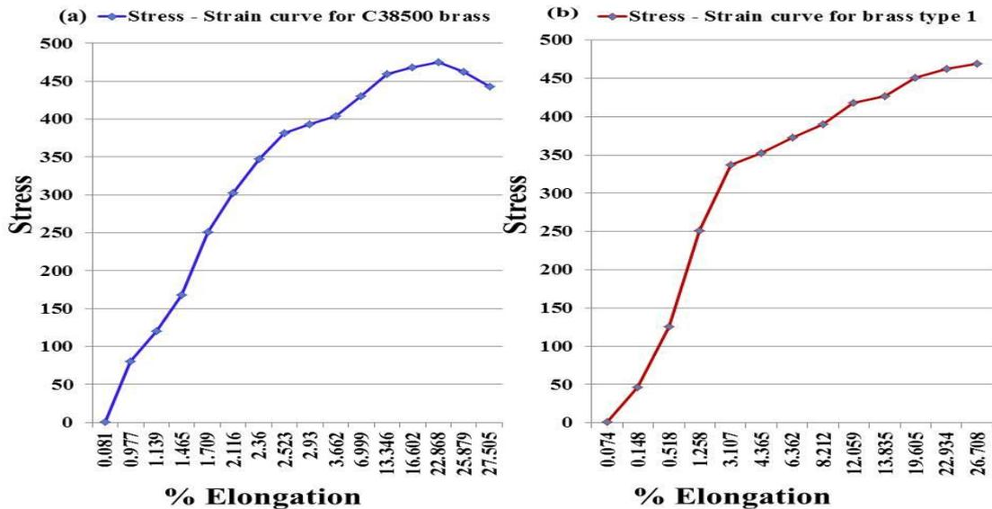
Figure 8. Typical stress–strain curves for (a) C38500 alloy; (b) brass type 1 alloy at strain rate of  $1.3 \times 10^{-4} \text{ s}^{-1}$ .
