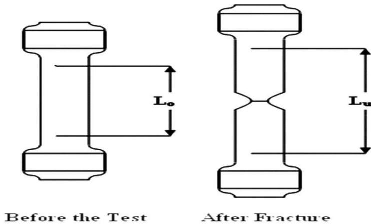
Figure 2. Change in length of a specimen after fracture.
