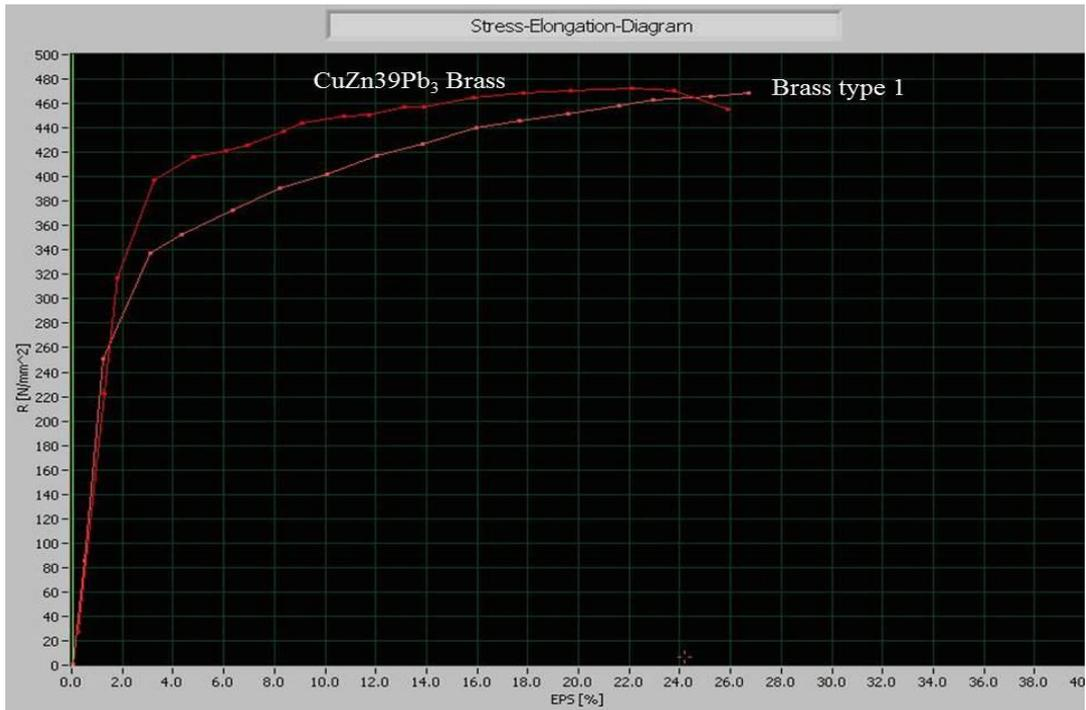
Figure 10. Comparative study of stress–elongation graph for C38500 brass alloy and brass type 1 alloy
