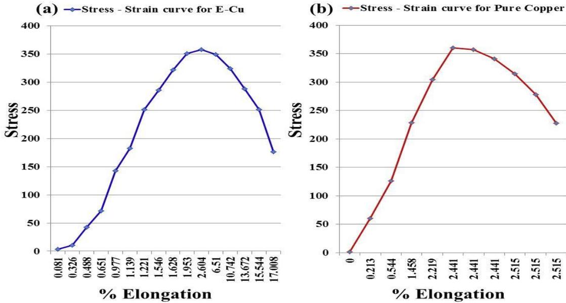
Figure 7. Typical stress–strain curves for (a) E-Cu alloy; (b) pure copper alloy at strain rate of  $1 \times 10^{-4} \text{ s}^{-1}$ .
