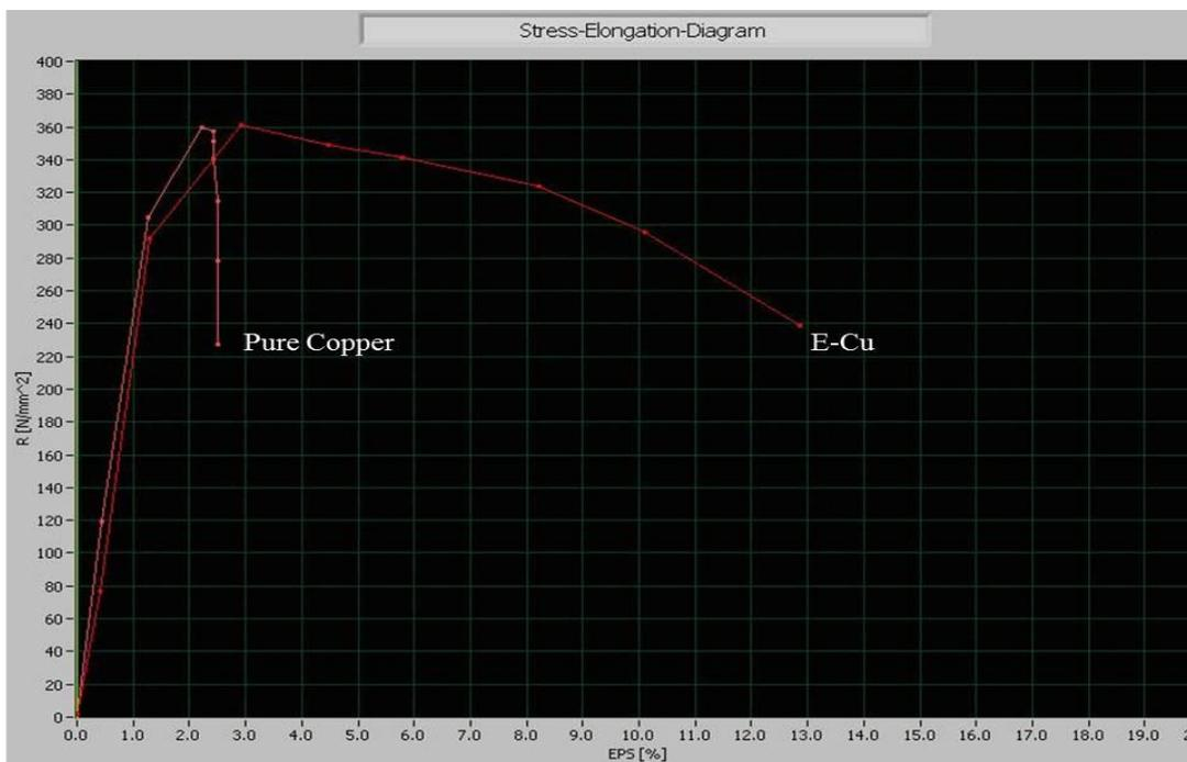
Figure 9. Comparative study of stress–elongation graph for E-Cu alloy and pure copper alloy.
