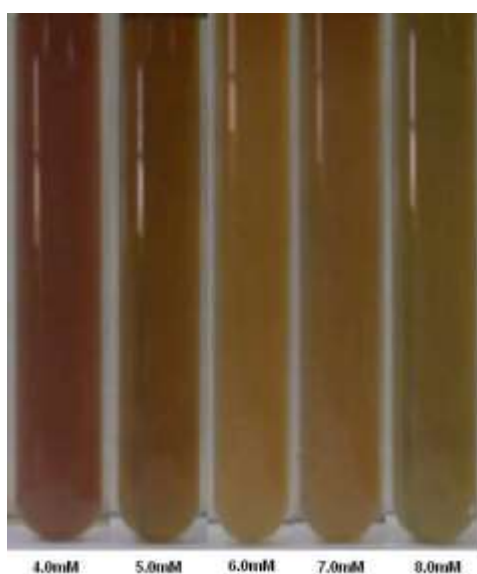
Figure 1. The final colour of Ag nanoparticles solution as a function of trisodium citrate dihydrate concentrations.
