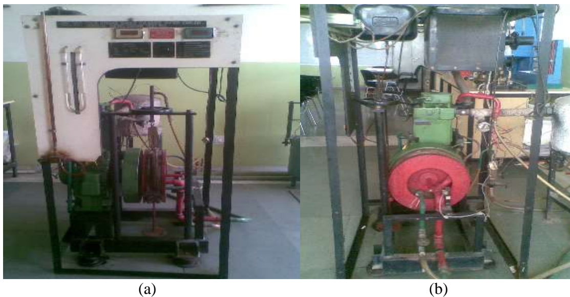
Figure 4. (a) Single cylinder diesel engine, (b) Rope brake dynamometer.
