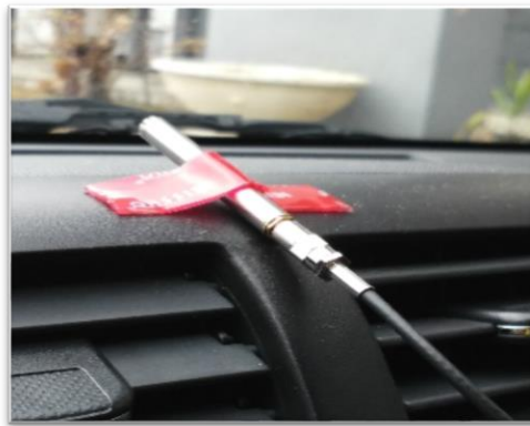
Figure 2. Microphone Placement: Front Dashboard
