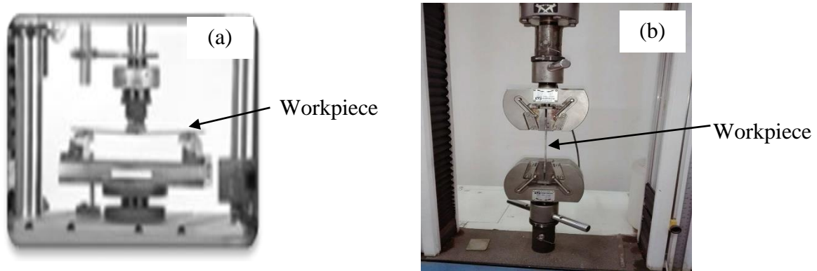
Figure 3. Picture of (a) flexural and (b) tensile tests set up with a workpiece.
