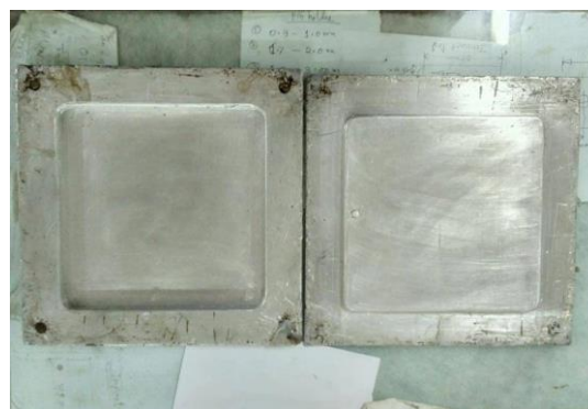
Figure 1. Picture of die used to prepare composites.
