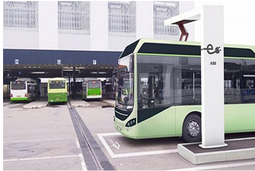
Figure 4. Quick electrobus charge (Luxemburg).
