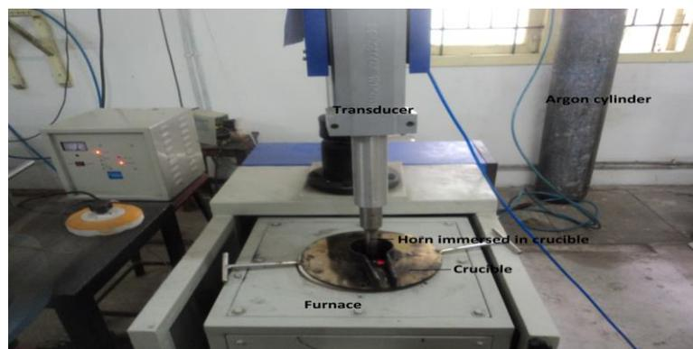
Figure 1. Ultrasonication assisted casting setup.
