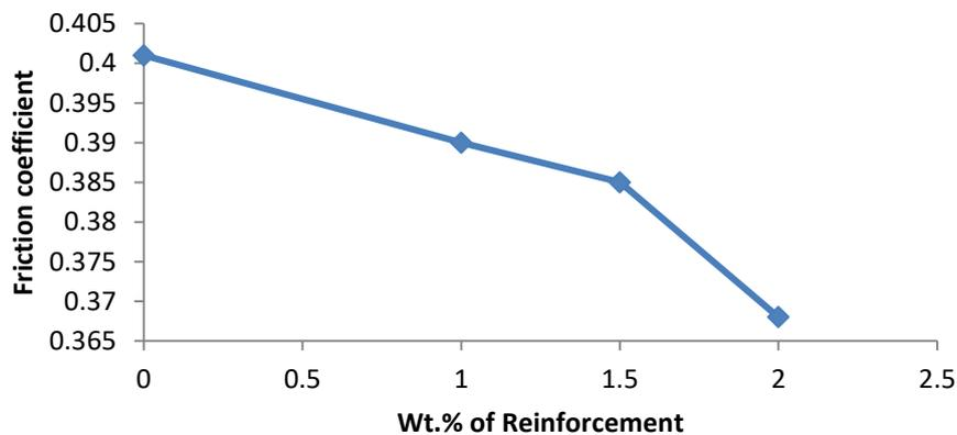
Figure 10. Friction coefficient Vs Wt.% of reinforcement
