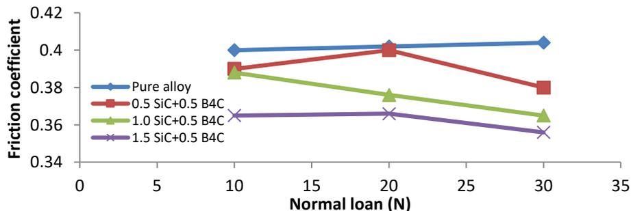
Figure 11. Friction coefficient against normal load.
