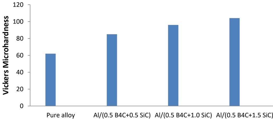
Figure 6. Microhardness Vs Wt.% of hybrid reinforcement.
