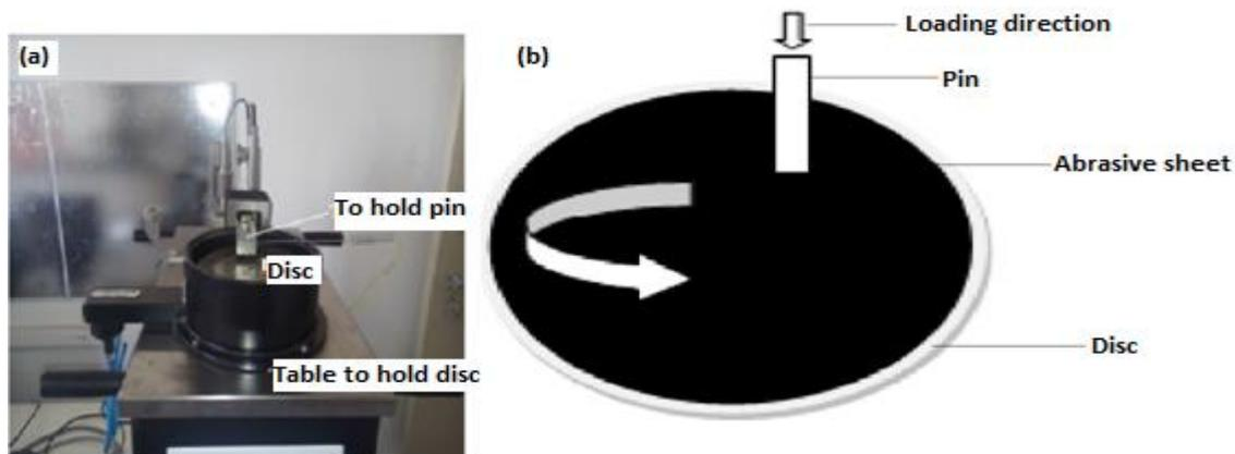
Figure 3. (a) Pin-on-disc tribometer (b) Schematic representation of abrasive wear test.
