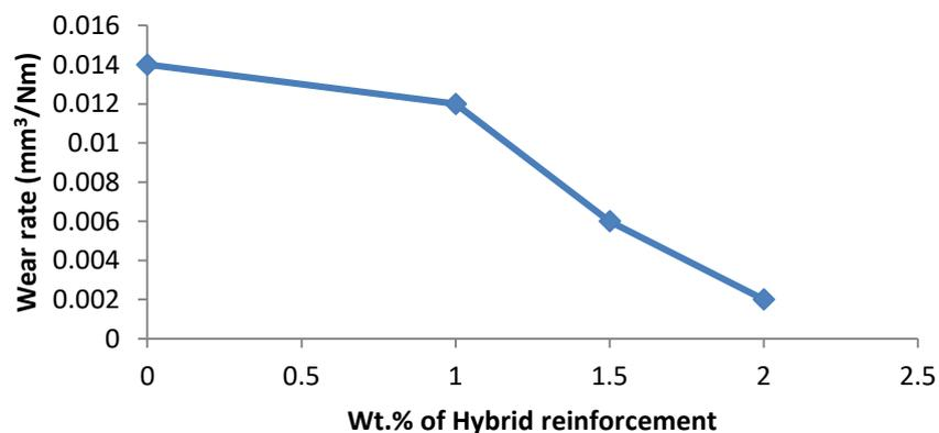
Figure 7. Wear rate Vs Wt.% of reinforcement
