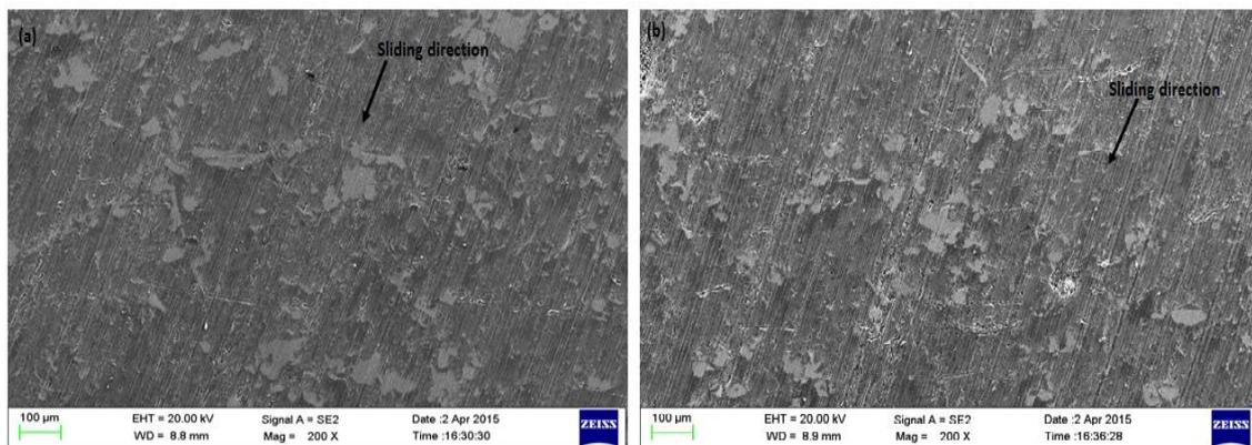
Figure 13. Worn surface FESEM images of Al/(0.5 Wt.% B<sub>4</sub>C+1.5 Wt.% SiC) nanocomposite (a) at 10 N (b) at 30 N.
