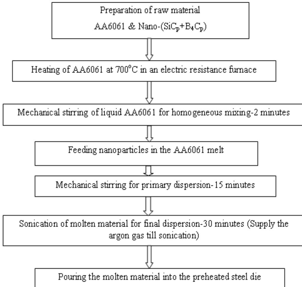
Figure 2. Procedures for manufacturing hybrid nanocomposites by ultrasonication assisted casting process.
