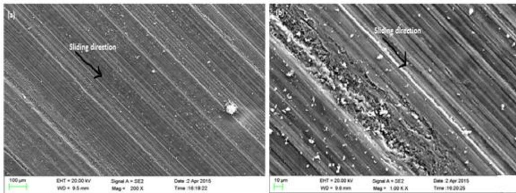
Figure 12. Worn surface FESEM images of Al alloy (a) at 10 N, 200 X magnification (b) at 10 N, 1000 X magnification.
