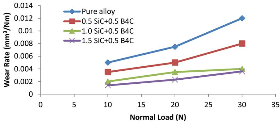
Figure 8. Wear rate against normal load.
