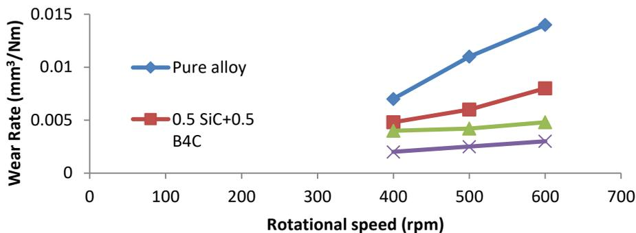
Figure 9 Wear rate against rotational speed.
