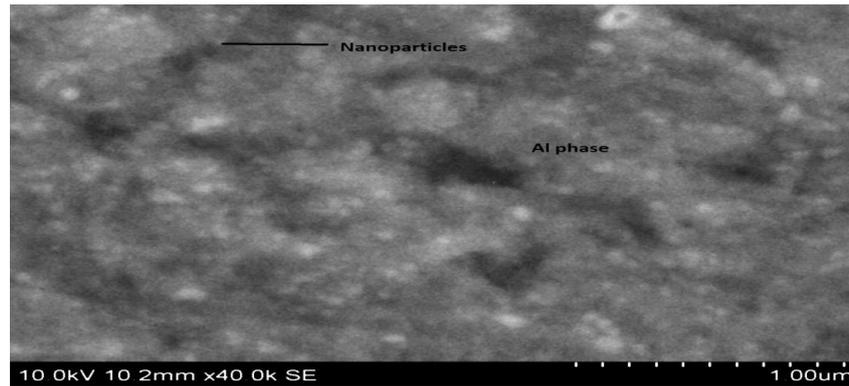
Figure 4. SEM image of a nanocomposite.
