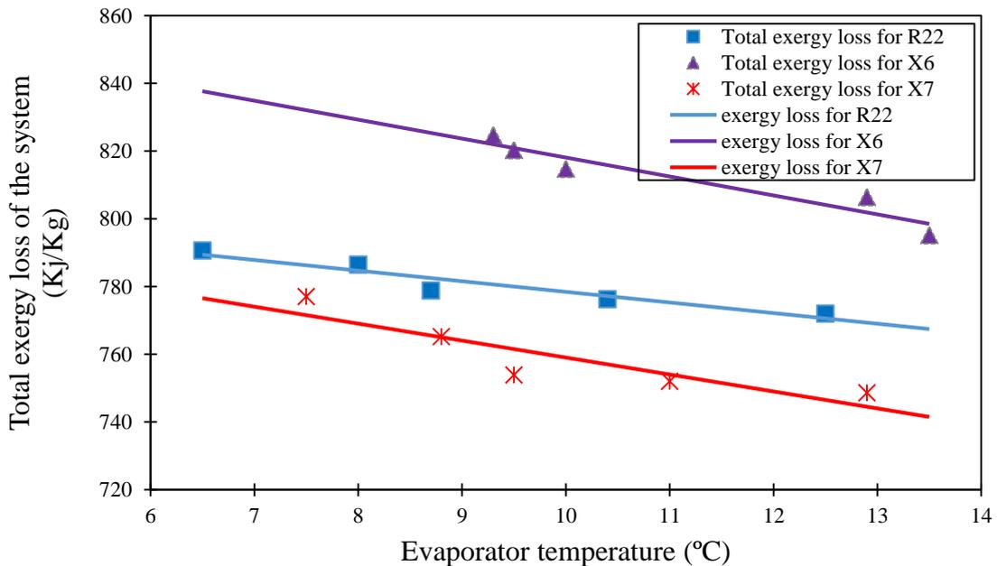
Figure 8. Change in exergy loss with evaporator temperature.
