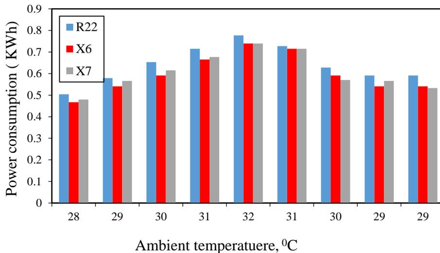
Figure 3. Variations of power consumptions using R22, X<sub>6</sub> and X<sub>7</sub> at different ambient temperatures.
