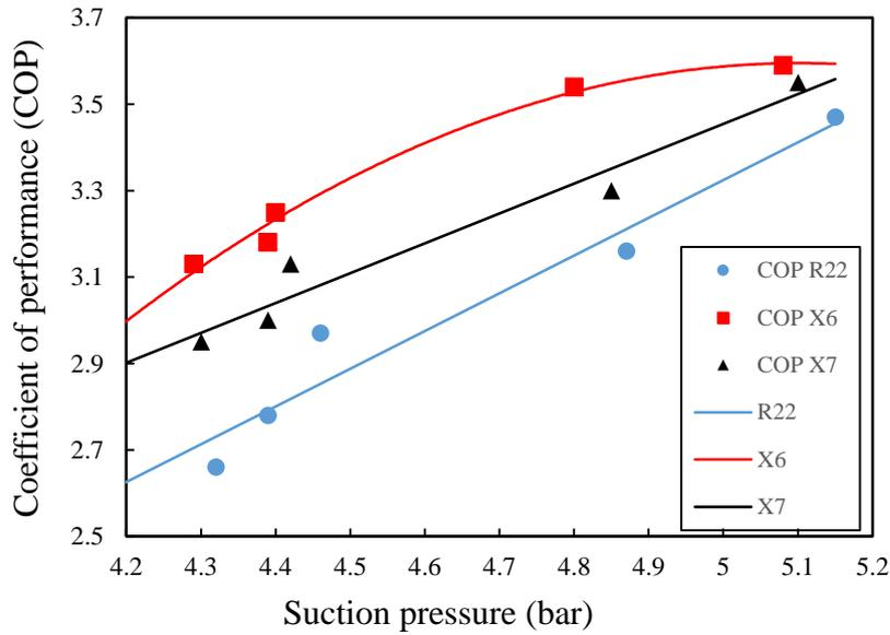
Figure 4. Variation in COP with evaporator pressure.
