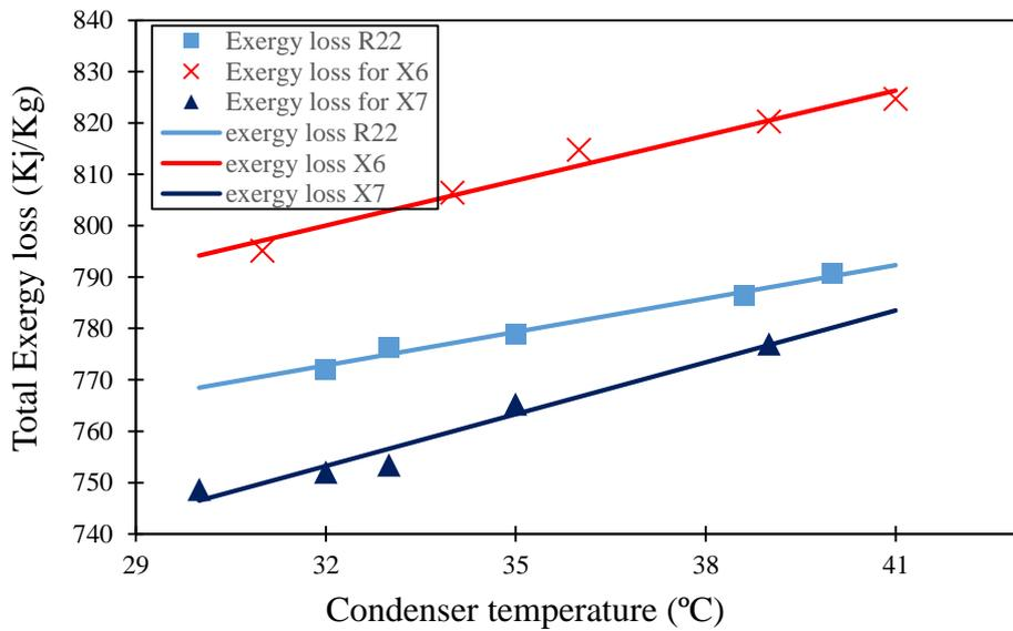
Figure 9. Exergy loss developing with condenser temperature.
