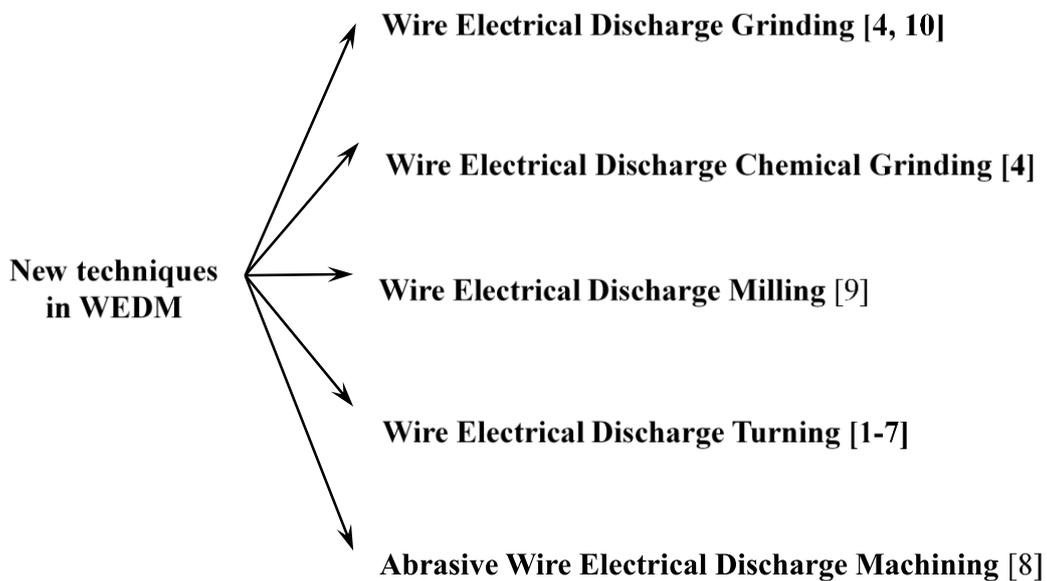
Figure 3. New techniques in WEDM process.
