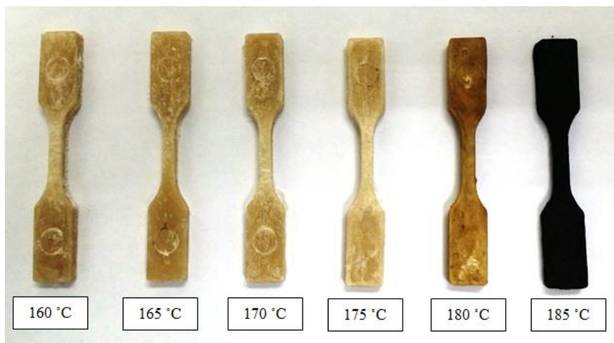
Figure 9. PLA tapioca resin biopolymer tensile test samples produced by injection moulding method.
