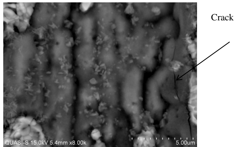
Figure 3. SEM image of sample sintered at 900°C for 90 mins.
