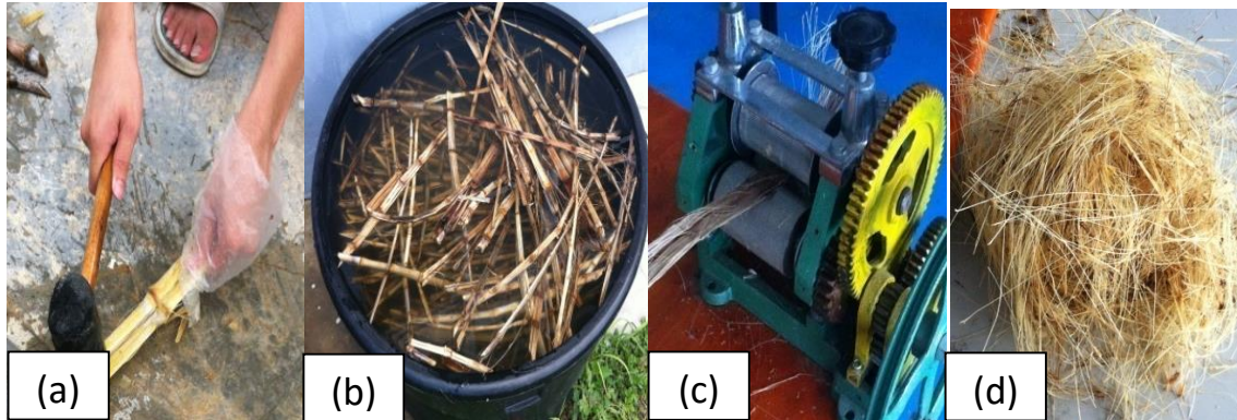
Figure 1. (a) Stem is beaten with a mallet, (b) soaked stems, (c) roll-out machine to separate fibres, and (d) extracted Napier grass fibre to be dried.
