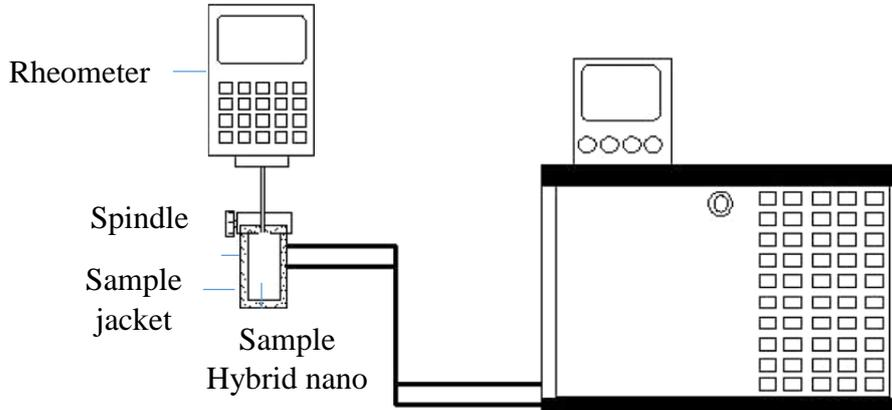
Figure 2. Viscosity measurement with the Brookfield Rheometer.
