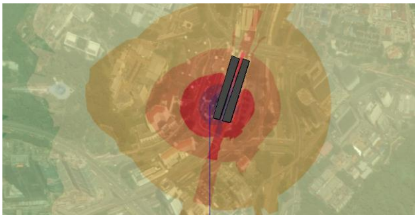
Figure 5. Noise mapping for Kuala Lumpur Station
