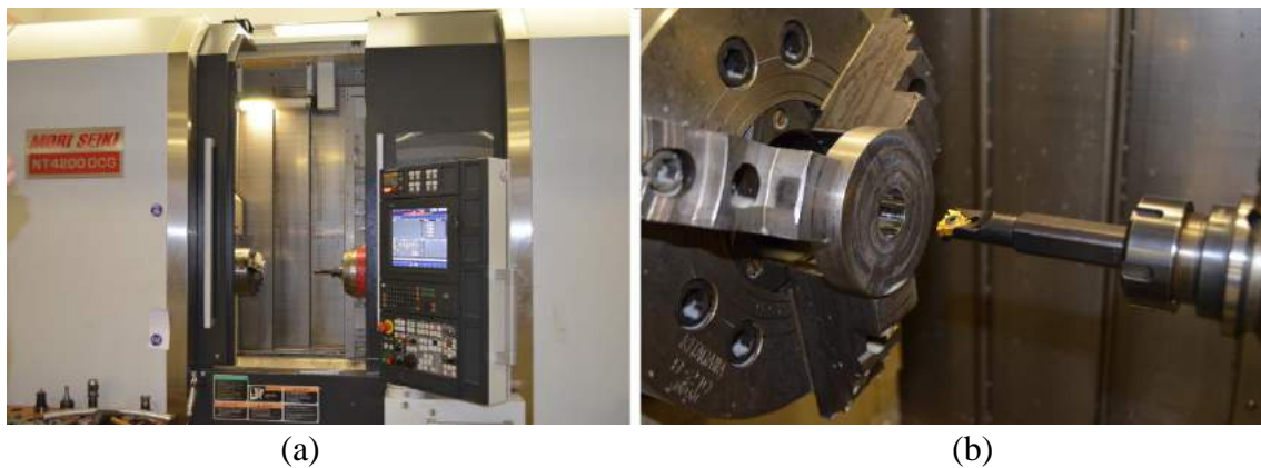
Figure 6. (a) Mori Seiki NT- 4200 DCG/1000S mill turn center; (b) workpiece and tool.
