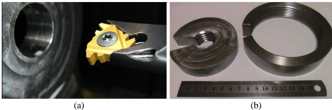
Figure 7. (a) Insert S32×4 and; (b) work pieces of 32 and 100 mm thread diameters.
