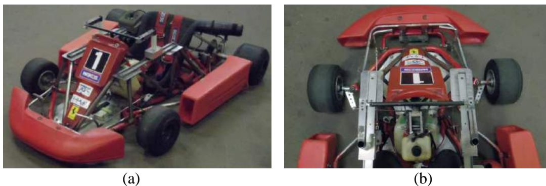
Figure 5. Racing kart with TLS steering system (a) overview and; (b) steering components.
